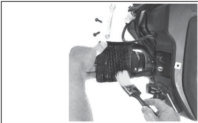
Figure 10. Cleaning Oil Cooler.
